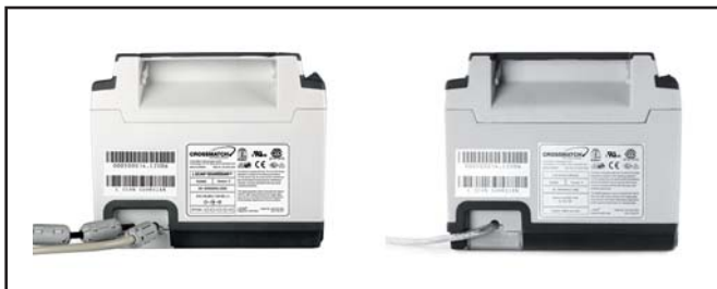
Guardian with USB interface (left) and Guardian with Firewire connection (right).
