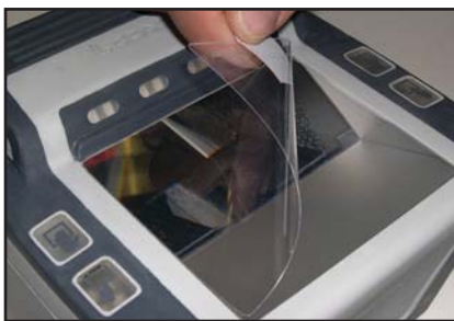
Silicone membranes are easy to replace on Cross Match livescan systems.
