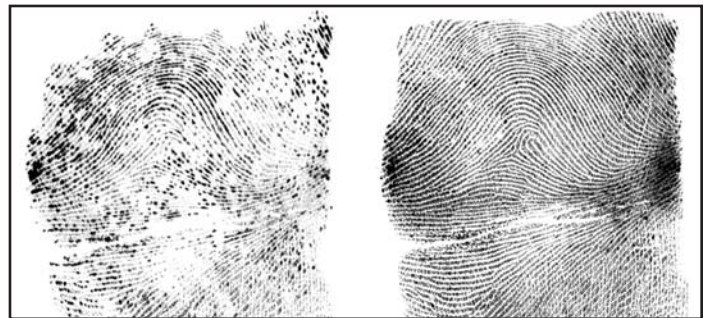
Livescan screen shots showing a comparison of fingerprint images taken both with (right) and without (left) the silicone membrane.
